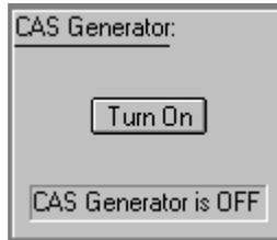
In this mode, the CAS generator can be turned on or off by clicking the center button. However, for the talk-off testing, the generator must be left off.
