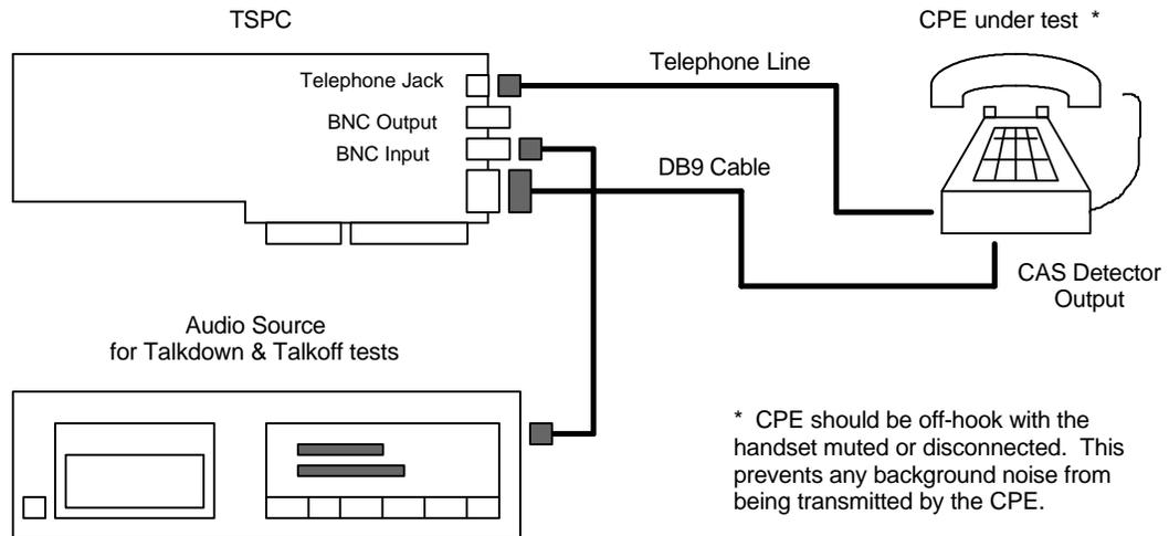
Figure 1: Test setup A
