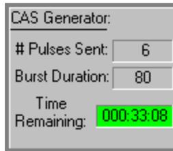
The number of pulses received by the data logger should match the number of CAS bursts sent. The test can be halted by pressing the Stop button on the timer, or the test reset by pressing the Reset button. The timer will normally stop once all of the CAS bursts have been sent. Then the "CAS Pulse Analysis" window can be displayed, showing all of the results of the test.
