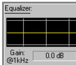
Once again, record the ASL level of each tape. Then similar to the talk-down and near-end talk-off tests, the desired ASL level can be set by adjusting only the gain of the equalizer. Since the ASL levels of each tape are now recorded, they do not need to be measured again.
