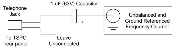
Note: In this setup, if the frequency counter and PC that contains the TSPC are not **both** properly connected to earth ground, a large amount of 50/60 Hz hum noise can effect the measurements.
