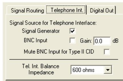
The Balance Impedance setting is used by the AI-7280 only when routing the telephone interface receive signals to the BNC output connector or to the measurement meter. In order for the AI-7280 to separate the receive signals (sent from the TE), from the signals
