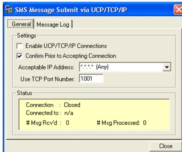
By enabling the TCP/IP connections and setting the desired IP address and port number, the TRsSim software begins listening for UCP messages. The **Message Log** tab records changes in the TCP/IP connection status and the contents of any UCP messages received.
