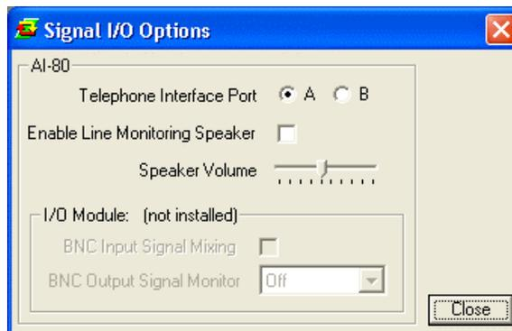
The two top buttons allow either the telephone interface port A or B to be used while the check box just below enables the built-in speaker for monitoring the telephone line. If the AI-80 is equipped with an I/O module, the BNC input connector can be used to inject signals onto the telephone line. In addition the BNC output connector can be used to monitor various signals by the selection of the drop-down list box.
