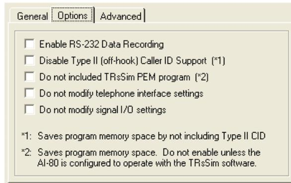
If the Data Recording option is enabled, the AI-80 outputs data from its RS-232 port during a SMS session. A special program called SmsMonitor is freely available from the TRsSim installation CD or our web site that decodes the data output. It shows the contents of any SMS messages sent by the TE.
