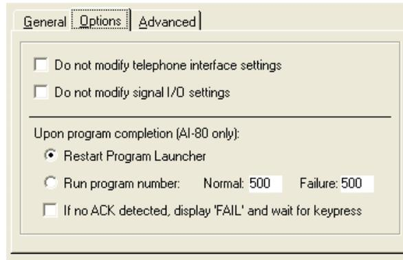
Normally the program created will configure the AI-80's or AI-7280's telephone interface settings and signal I/O settings to match the current TRsSim settings. However, by enabling the top two check boxes, the Caller ID program created does not change the device's telephone interface or signal I/O settings respectively.
