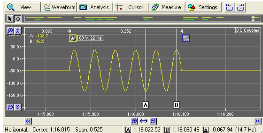
If vertical cursors are enabled, the point at which the cursor intersects the waveform is displayed in the top left corner of the graph. In the example figure above, cursor A measures a waveform voltage of -132.7 volts, while cursor B measures 36.5 volts.
