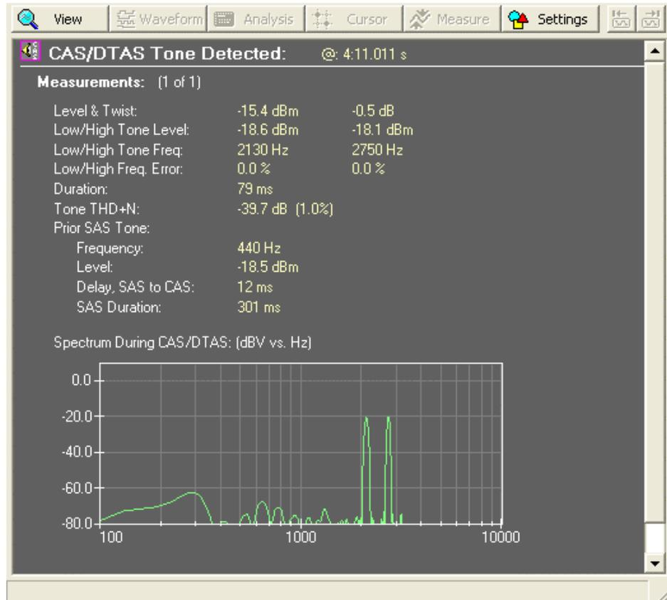
If a SAS (subscriber alerting signal) was detected prior to the CAS/DTAS tone, the analysis attempts to extract its frequency and level. In the example above, a SAS tone was detected with a duration of 301 ms and ending just 12 ms before the CAS/DTAS tone started.
