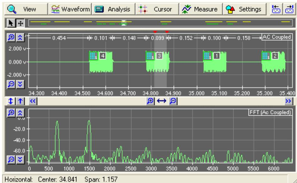
In this split display, the horizontal pan and zoom buttons are used to control both the top waveform graph and the bottom FFT graph, though not at the same time. The buttons modify the horizontal settings for the last graph selected. To change which graph is selected, click the left mouse button anywhere on the graph.
