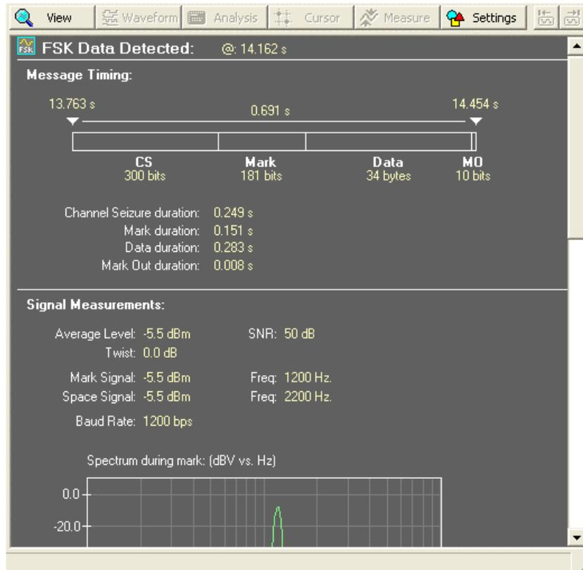
Note that depending on the message bit pattern, some measurements may not be possible. For example, if an insufficient number of consecutive zero bits are contained within the message, an accurate space frequency and space level measurement can not be made.
