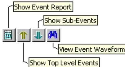
Depending on the selected event, not all of the buttons may be visible. The two outside buttons are used to display either the event waveform or event details in a Data Recorder window. The two inner buttons navigate the event hierarchy. Some events may be composed of sub-events. An example of this is DTMF dialing. The following figure shows an event of DTMF dialing. The details indicate that the digits "6049454312" were dialed with a total duration of 3.142 seconds.
