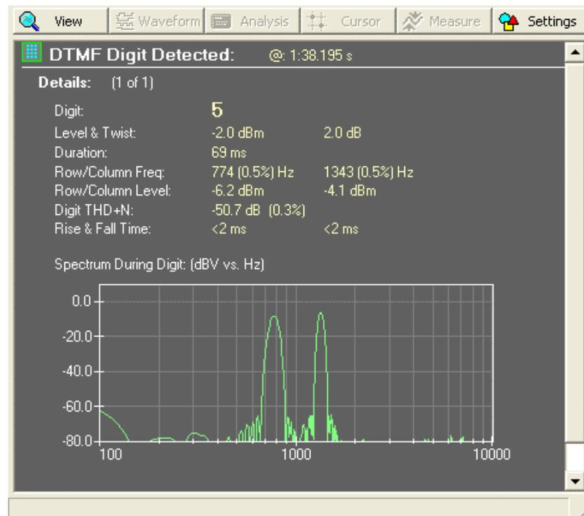
If any signal measurements are found to be outside the specified DTMF dialing limits, warnings are displayed in the report.
