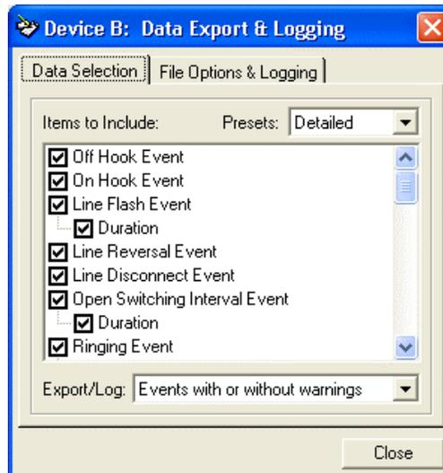
The first of two tabs sets the event filter. Any event listed with a checkmark beside the name is exported and logged (if logging is enabled). In addition, some events have the option to export/log measurement or analysis data if the appropriate box is checked. The
