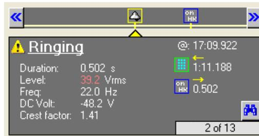
Events that have warnings, display a 'warning' icon to the left of the event name in the control panel. In addition, any measurements that caused the warning are highlighted in a red color.
