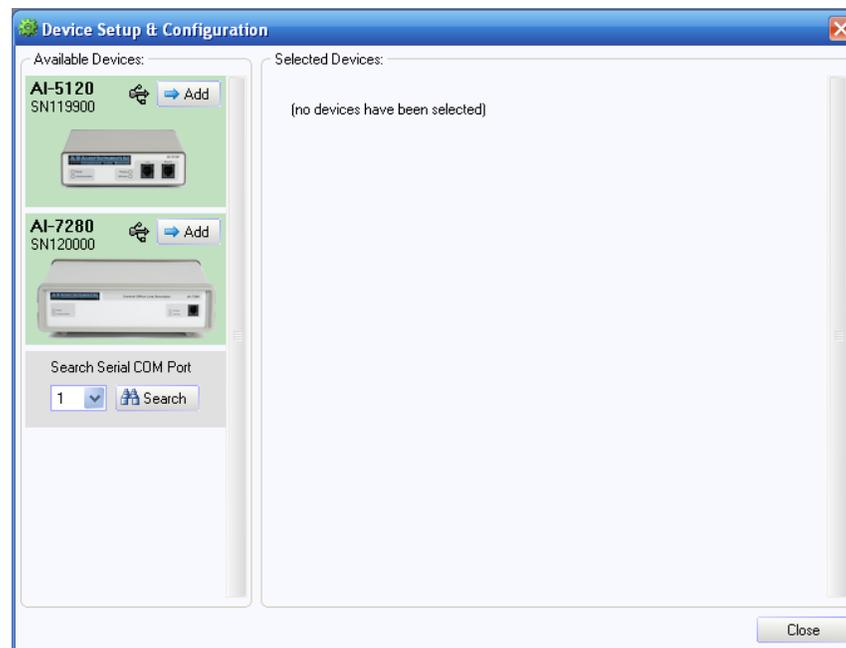
Available devices connected via USB are automatically displayed. However for devices connected via a RS-232 serial port, they must be discovered manually by clicking the **Search** button.
