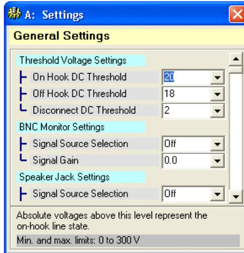
The various parameters are grouped into different categories. To modify any of the settings, simply click the mouse on the text box to the right of the parameter name and enter or select the new setting value. Displayed at the bottom of the window is additional information regarding the selected parameter along with minimum/maximum limits (if applicable). As only a few of the parameters are visible at any one time, use the scroll bar on the right side to slide the list either up or down.
