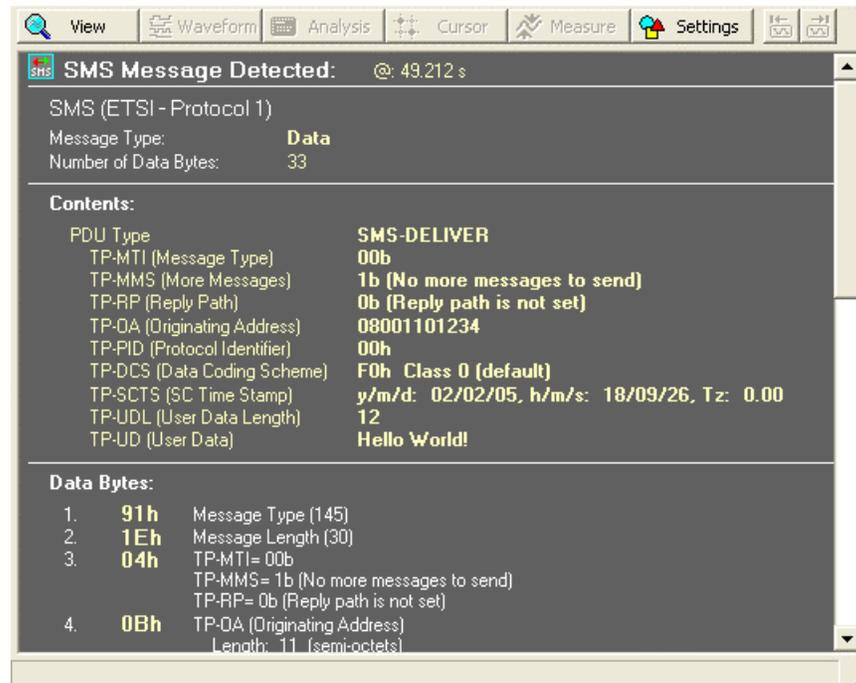
The results of the data layer report contain the same information as detected Caller ID or SMS events. The only significant difference when performing the **FSK - Data Layer** analysis is that the source of the data can be any waveform. This includes waveforms recorded by the AI-5120 when FSK events are detected, or waveforms imported from files.
