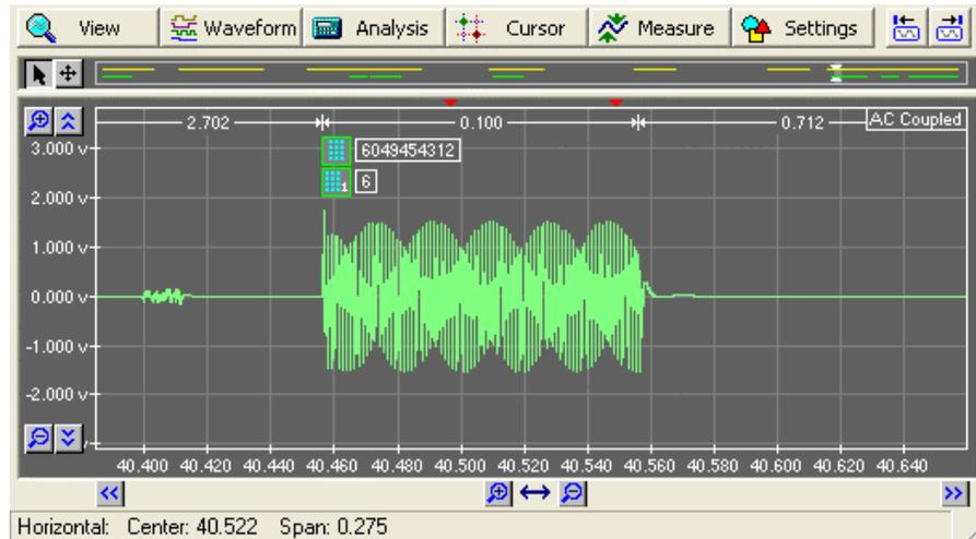
Waveforms are display on a graph using time for the horizontal axis and voltage for the vertical axis. In this example, the DTMF digit starts at approximately 40.46 seconds with a duration of 100 ms. Event icons and timing markers above the waveform indicate the type of event along with timing relationships to other events. Both of these graphical tools may be turned off by using the **View** button menu.
