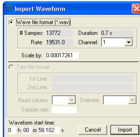
If a text file is read, an attempt is made to extract the column containing the waveform samples, delimiter character, and sample rate. These may be changed if incorrect by entering a new value for the field.
