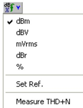
The bar graph scale reflects the current unit settings, except for the units of mVrms. In that case the bar graph is calibrated to dBV. The dBr and % units are relative to a defined reference level. The reference level can be set to the current level reading by choosing the **Set Ref.** menu selection. As an alternative, it can be specified in Vrms from within the **Level Meter & Filter Settings** window.
