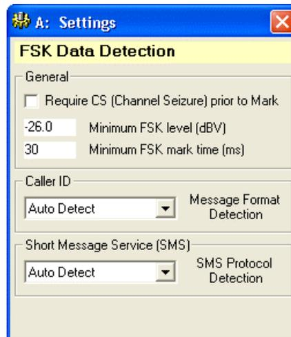
The three settings grouped in the **General** category apply to all FSK messages. If the "Require CS" setting is checked, then all FSK message require a channel seizure signal to be present prior to the mark signal. Channel seizure is defined as an alternating one/zero bit pattern with a duration of at least 50 ms (60 bits).
