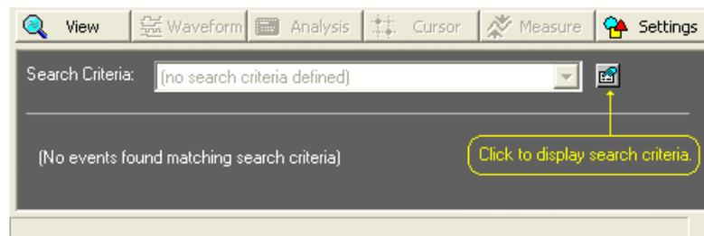
Many different search criteria can be defined, as each one is identified by a name given to it when created. When the search criteria window is first displayed, there are no criteria defined. As such, the first step is to click the **New** button in order to create a new search criteria. A window appears requesting a unique name for the criteria. Once a name is entered and the **OK** button clicked, a search criteria can be defined.
