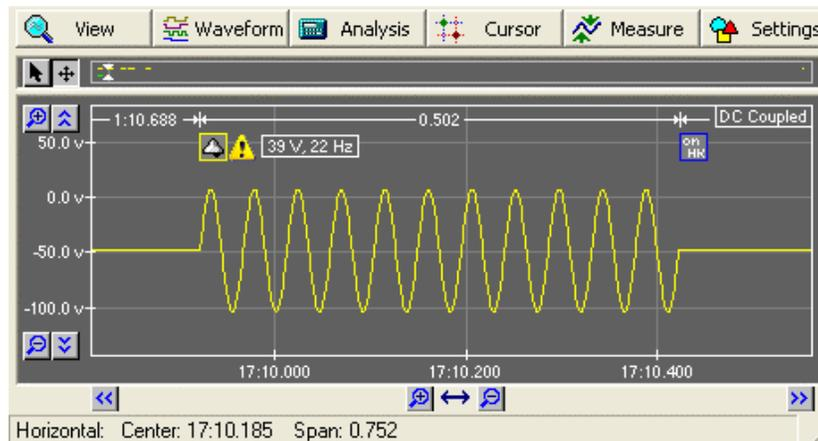
The ringing event is also flagged in the event listing. Any warning messages associated with an event are displayed beneath the measurement values.
