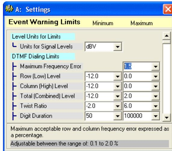
The first setting determines the unit system used to define all event limits that relate to signal levels. This may be either dBm (default), dBV, or mVrms.
