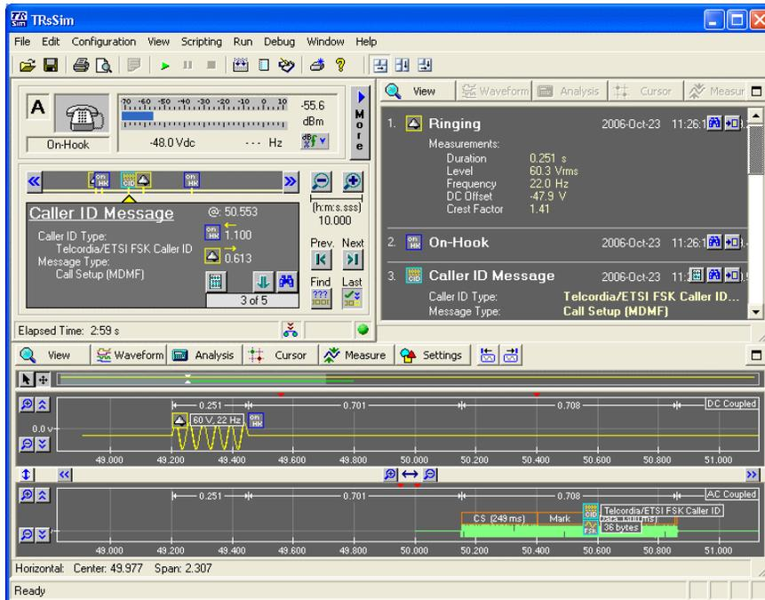
In the above figure, the AI-5120 has detected ringing followed by a FSK Caller ID transmission. The top right window lists each event detected, while the bottom window displays the recorded waveforms. As additional events are detected by the AI-5120, the listing of events is automatically updated and any new recorded waveforms are displayed.
