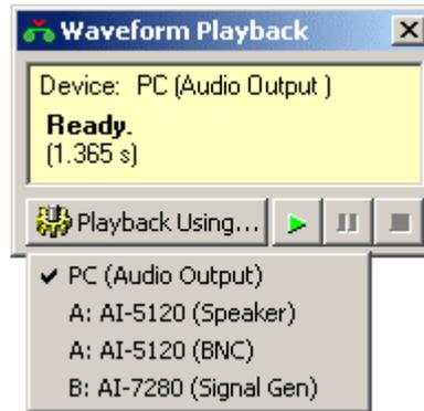
After selecting the playback device, the waveform is loaded into the device. Once finished, click the play button (green triangle) to start playback.
