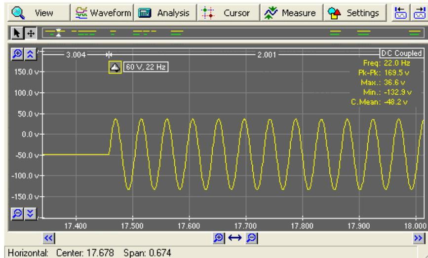
When the Data Recorder window shows large time spans, the measurement functions may not be accurate. This is because when greatly zoomed out, the measurement functions only operate on a subset of the all the waveform's data points. When this occurs the character '\*' is displayed following the measurement value. For accurate measurements the time span should be reduced until the '\*' character is no longer shown.
