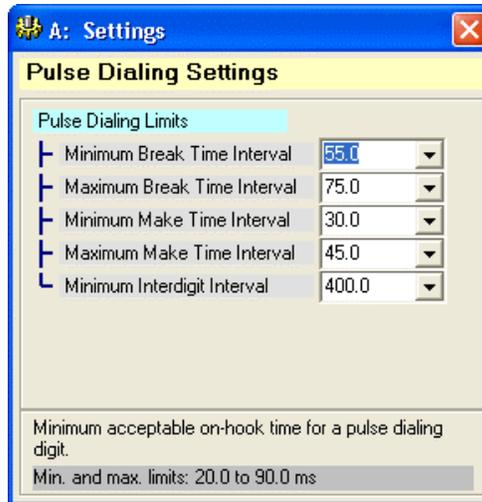
The minimum and maximum break time limits define the range of time the telephone line must be in the on-hook state. The make time range then defines the amount of time required between the on-hook pulses. The number of pulses determines the dialed digit (from 1 to 10, 10 representing digit zero).
