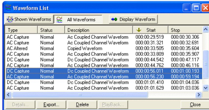
The two buttons at the top of the window, labeled **Shown Waveforms** and **All Waveforms** toggle between listing only the currently visible waveforms or all of the recorded waveforms. By selecting a waveform in the list, it can be displayed on the Data Recorder window by clicking the **Display Waveform** button. In addition, the buttons at the bottom of the window may be used to alter the selected waveform details, export the waveform(s), delete the waveform(s), or playback the waveform(s).
