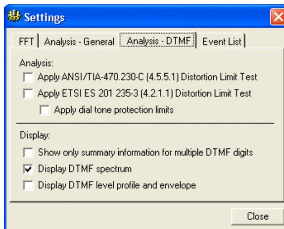
The last three settings affect how the analysis data is displayed for the DTMF reports. The first setting, if enabled, limits the report to only summary information, while the following two enable or disable the display of the DTMF spectrum and level profile.
