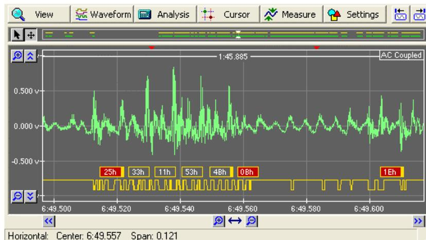
The FSK decoder waveform at the bottom of the display shows either a high (mark) or low (space) state. Any bytes detected are shown just above the decoder output. Bytes that are displayed with a red background color indicate that at some time during the byte,
