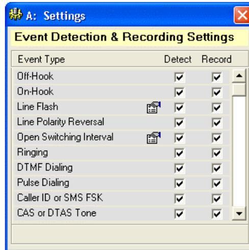
Events will be detected and time stamped by the AI-5120 if a checkmark is present in the **Detect** column. The **Record** column indicates if any waveforms should be recorded once the event is detected. If an event is not enabled for detection, then it can not be enabled for recording.
