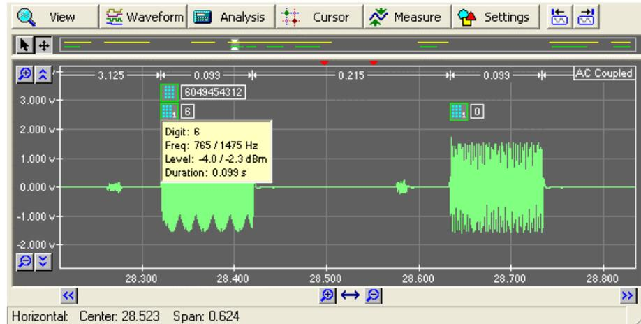
In addition to the event icons, timing lines are drawn at the very top of the graph. These timing lines correspond to the start time of events and the duration of events. In the example above, the timing lines display the duration of the two DTMF digits as well as their inter-digit time.
