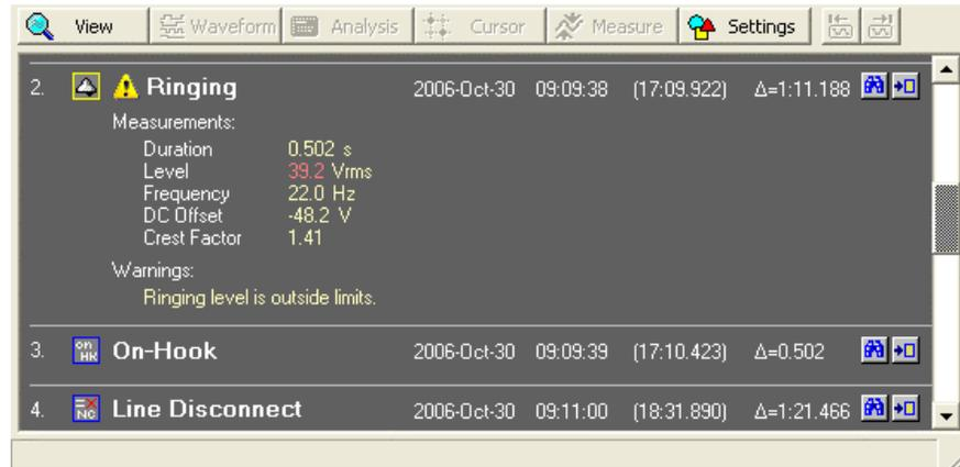
The Event List display in the Data Recorder window can be configured to only display events with warnings, or ignore all events with warnings. The event list filter controls are accessed by clicking the **Settings** button, followed by the **General Settings** command.
