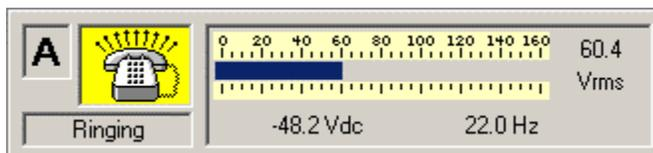
The units of level measurement during ringing are fixed at Vrms.
