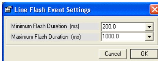
The Line Flash event has two additional settings. These set the minimum and maximum detectable flash time. Only line flashes with durations between these limits are detected by the AI-5120.
