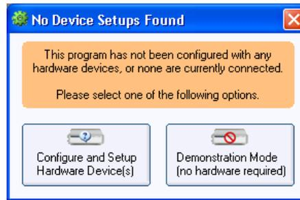
Click the **Demonstration Mode** button if you do not have any hardware connected to the PC and would like to evaluate the software. This bypasses the hardware setup and continues the process of loading the remaining software. By running in demonstration mode the software is unable to control any connected hardware; however the various software features and general user interface can be explored.
