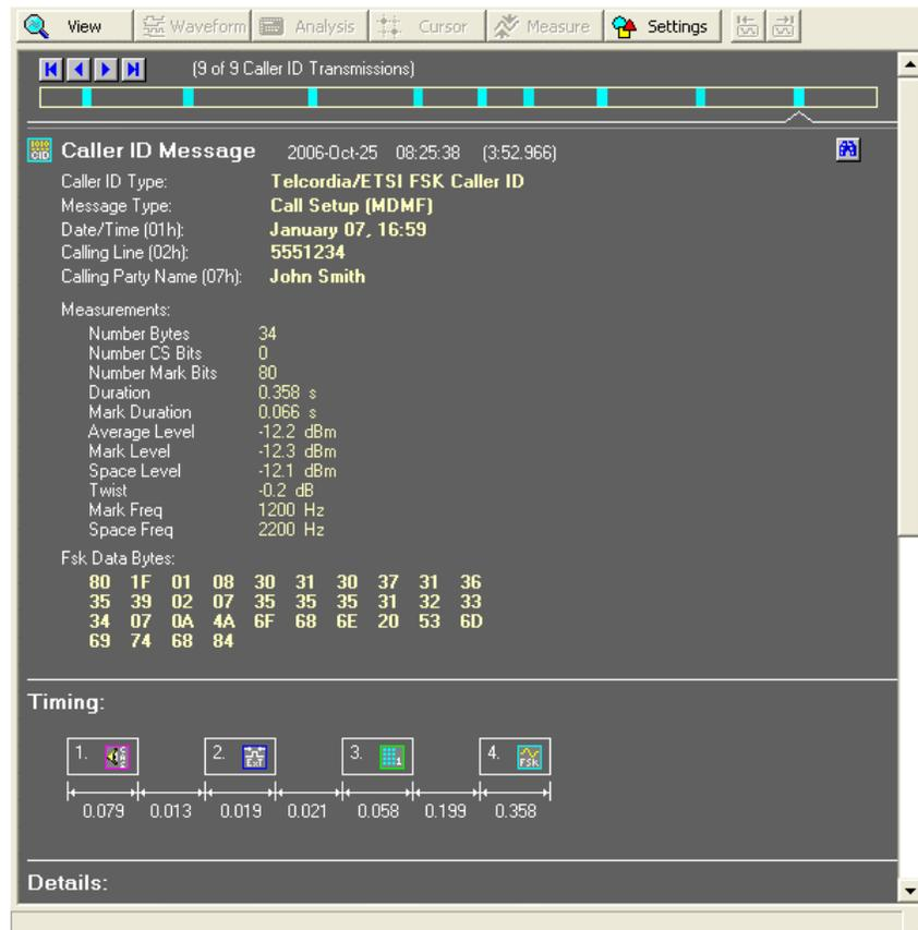
Below the displayed header is a summary of the selected Caller ID transmission consisting of three sections. The first section lists details on the Caller ID message contents as well as FSK waveform measurements and a listing of the decoded data bytes.
