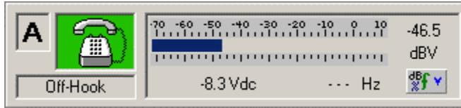
At low signal levels, no frequency measurement is returned. Only when the signal level exceeds 50 mVrms (-26 dBV) is a frequency reading displayed. The default signal level unit of dBm can be changed to either dBV, mVrms, dBr, or % by clicking on the units button just underneath the level reading.
