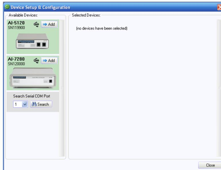
The above figure shows that two devices, an AI-5120 and AI-7280 are available to TRsSim. Select the desired device and add it to the list of selected devices, by clicking the **Add** button
