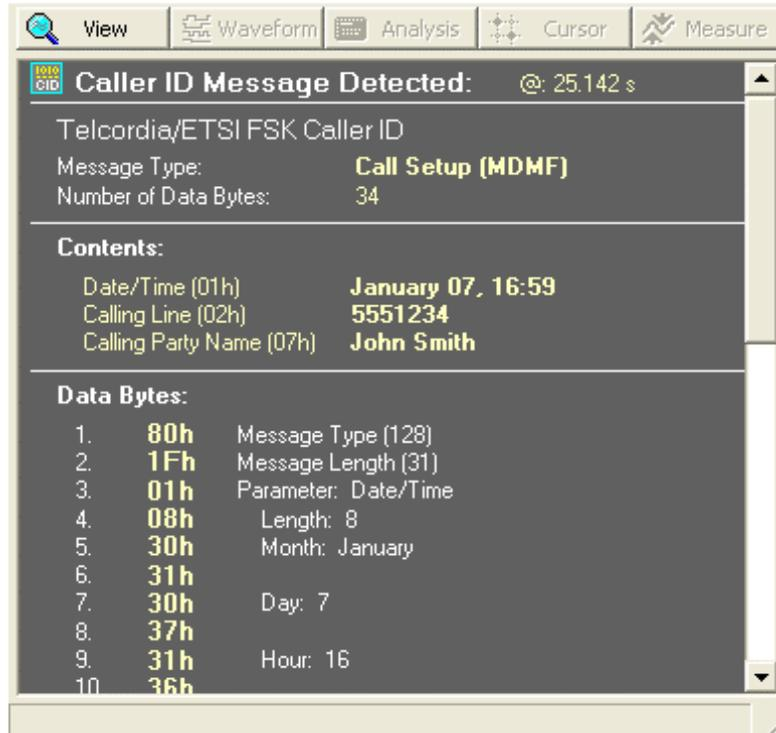
It provides more detailed information than possible on the main control panel. In the above example the contents of the Caller ID message along with the FSK byte values are displayed.
