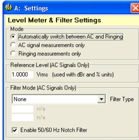
The level meter shown on the main control panel shows either AC signal measurements or ringing measurements. Normally the mode changes automatically when the AI-5120 detects ringing. The **Mode** selection shown in the above figure can be used for fix the measurements to either AC signal or ringing.
