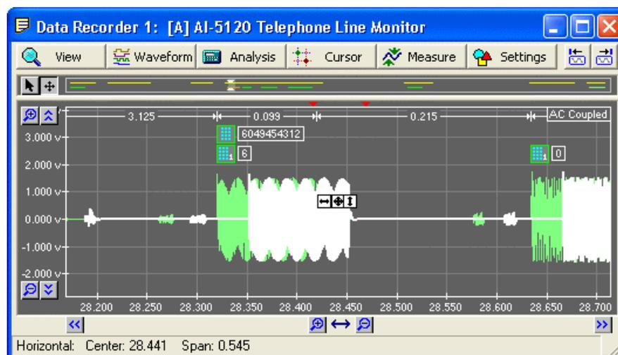
After panning the display to the desired horizontal position for the copied waveform, select the **Lock Position** command from the **Waveform** menu. This locks the copied waveform's time position on the graph. It now pans just like all the other waveforms shown.
