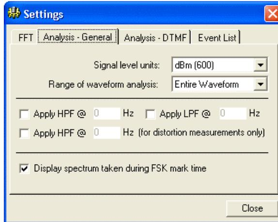
The next group of controls are used to enable optional low and high pass filters. If the corresponding check box is marked, a 4<sup>th</sup> order Butterworth low and/or high pass filter may be applied to the waveform before any analysis is performed. The corner frequencies of both filters are programmable between the range of 50 to 5000 Hz for the high pass filter and 100 to 10000 Hz for the low pass filter.
