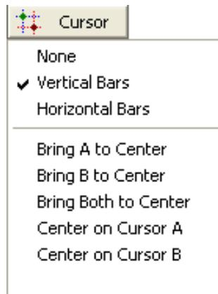
Cursors can operate in either a horizontal or vertical mode. To change modes, simply click the **Cursor** button and select the desired mode. In either mode, two cursors (labeled 'A' and 'B') are made available for measurements.
