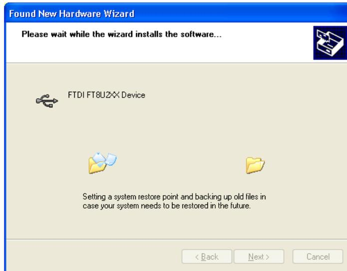
Once the installation is complete, the AI-7280 will be ready for use. The name for the USB driver is "FTDI FT8U2XX Device" so that when viewing the Control Panel's 'Device Manager' window, the AI-7280 is indicated by the "FTDI FT8U2XX Device" driver name.
