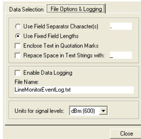
Note that if logging is enabled, the detected event is written to the log file only after a time delay of approximately 30 seconds.
