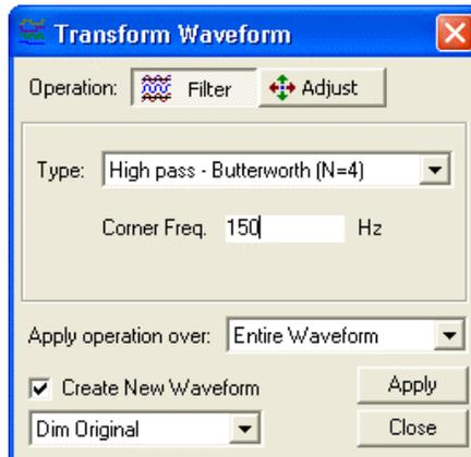
Two different types of operations may be performed. They are either filtering or adjusting the gain, offset, and time position of the selected waveform. The two buttons at the top of the window select the desired mode.
