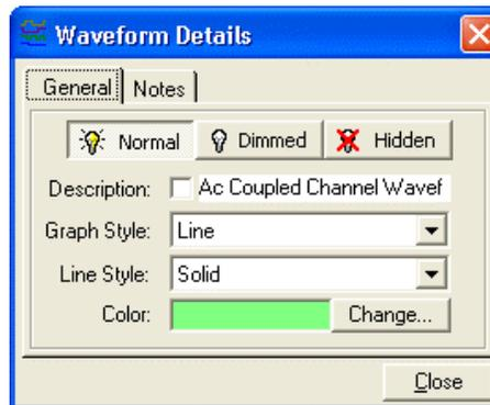
To add waveform notes, click the tab marked **Notes**. This displays a text area to enter notes linked to the selected waveform. Notes for any selected waveform are viewed by clicking the **Show Notes** command from under the **Waveform** menu.
