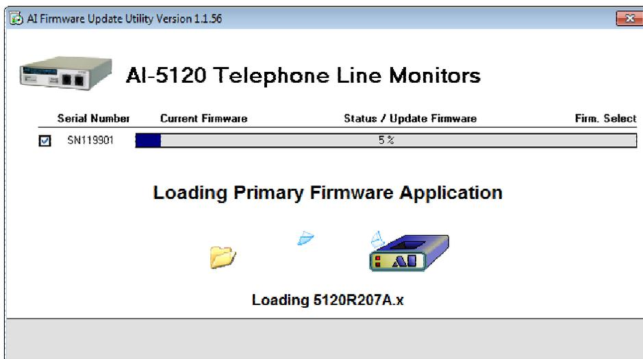
Once the update process is complete and no errors were detected, a green icon is shown to the left of the device information. If the update could not be completed due to errors, a message providing information on the error is displayed. Please contact us for assistance in resolving the error.
